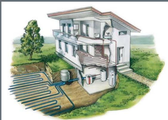
There are many ways of utilising ground heat, the most efficient of these is direct ground heat sourcing. Here, the heat pump's working medium circulates as a heat carrier directly in the flat-laid collectors.
